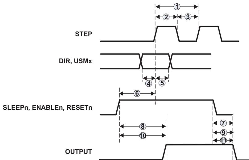
Figure 1. Timing Diagram
