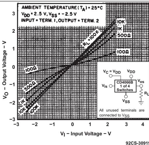
Figure 5. Typical ON Characteristics for 1 of 4 Channels
