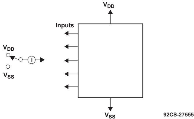
Measure inputs sequentially to both  $V_{DD}$  and  $V_{SS}$ . Connect all unused inputs to either  $V_{DD}$  or  $V_{SS}$ . Measure control inputs only.
