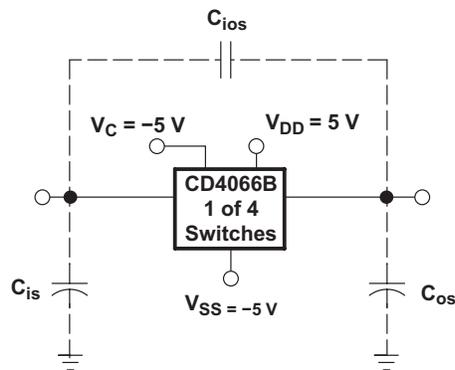
Measured on Boonton capacitance bridge, model 75a (1 MHz);
