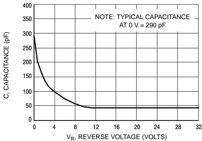
Figure 7. Typical Capacitance
