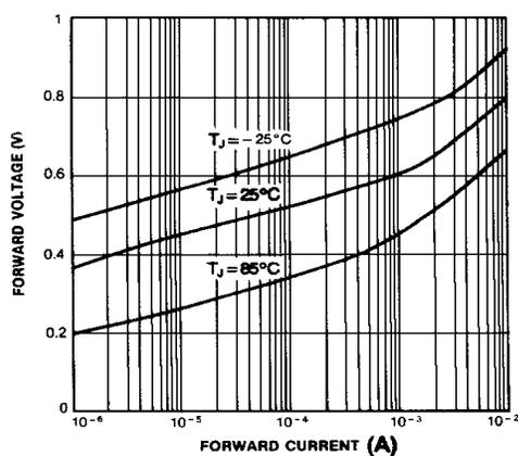
Figure 3. Forward Characteristics
