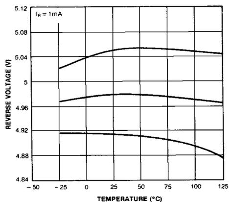
Figure 2. Temperature Drift
