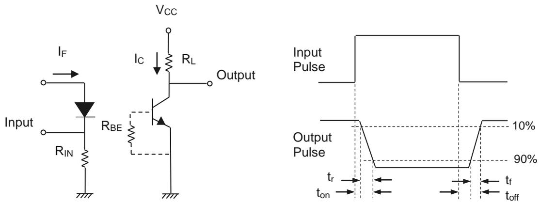
Figure 11. Switching Time Test Circuit & Waveforms
