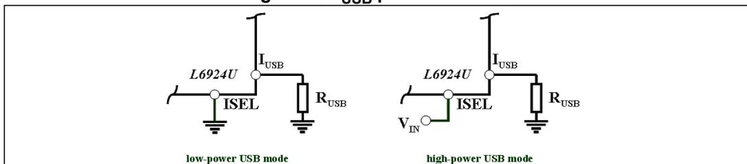
Regardless of the operation mode (AC adapter or USB), during the fast-charge phase the battery voltage increases until it reaches the programmed output voltage (4.2 V). A safety timer is also present. If the Fast-charge phase does not finish within the programmed time (see [Chapter 7.7: Maximum charging time on page 22](#)), a fault is given.
