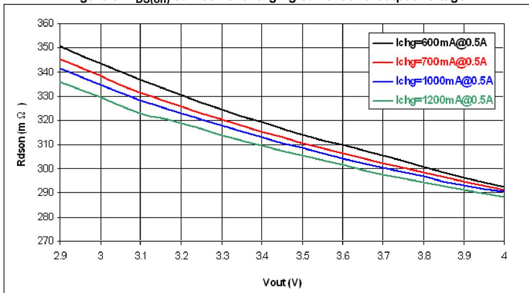
Neglecting the voltage drop across the charger ( $\Delta V_{MOS}$ ) when the device operates in this condition, its input voltage is equal to the battery one, and so a very low operating input voltage (down to 2.5 V) is required. The power dissipated by the device during this phase is:
