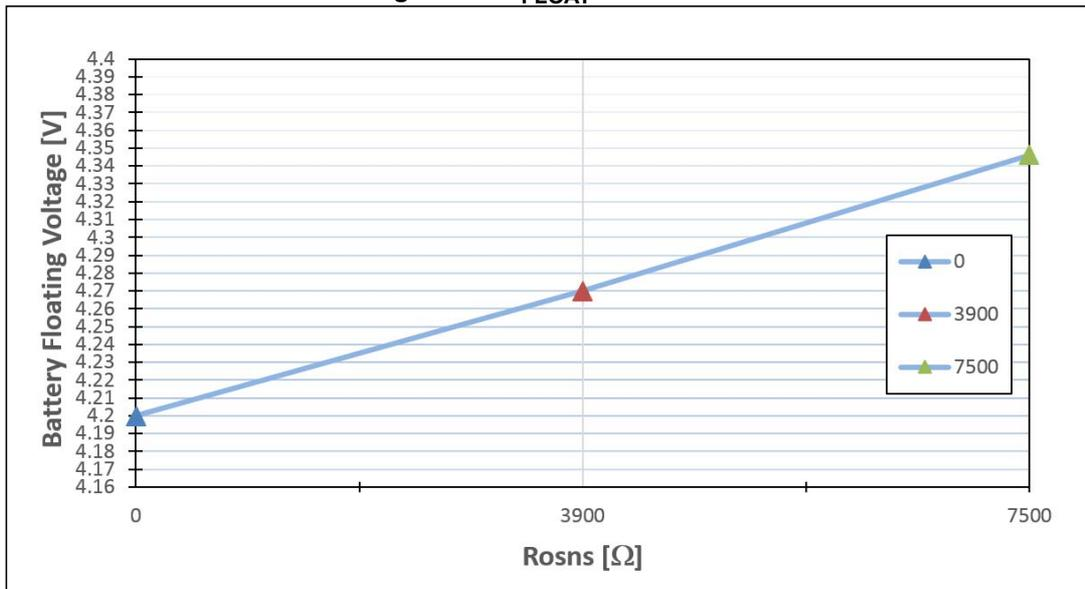
The L6924U works with the selected external components. The test results confirm that their behavior is in line with the design.
