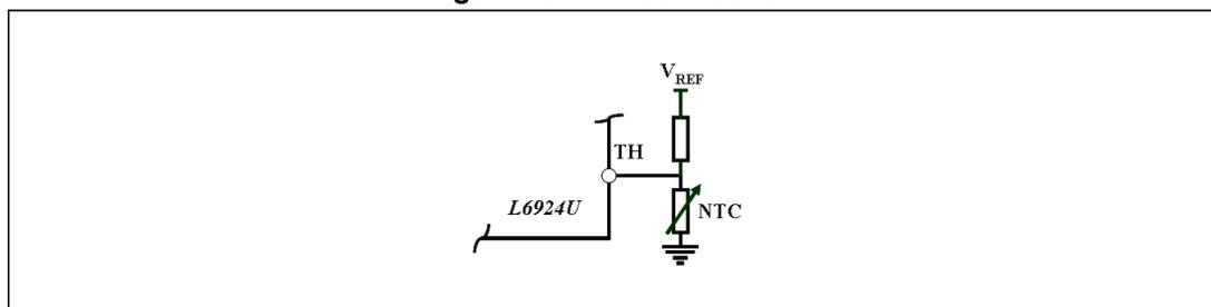
When the TH pin voltage rises and exceeds the  $V_{\text{MINTH}} = 50\%$  of  $V_{\text{REF}}$  (900 mV typ), the L6924U stops the charge, and indicates a fault by the status pins. The device re-starts to charge the battery, only when the voltage at the TH pin goes under  $V_{\text{MINTH\_HYS}} = 780$  mV (typ).
