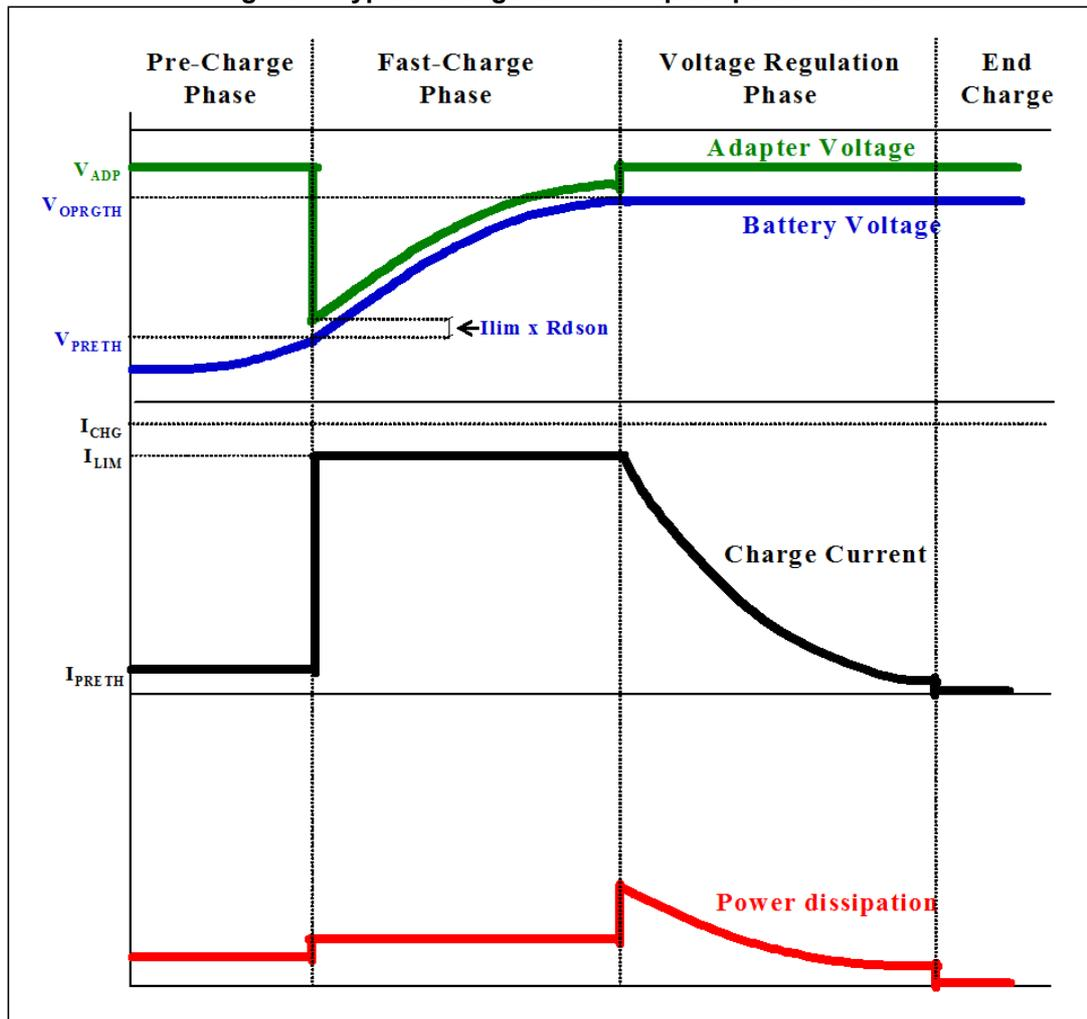
The big difference is due to the fact that the charge current is higher than the current limit of the adapter. During the fast-charge phase, the output voltage of the adapter drops and goes down to the battery voltage plus the voltage drop across the power MOSFET of the charger, as shown in the following equation:
