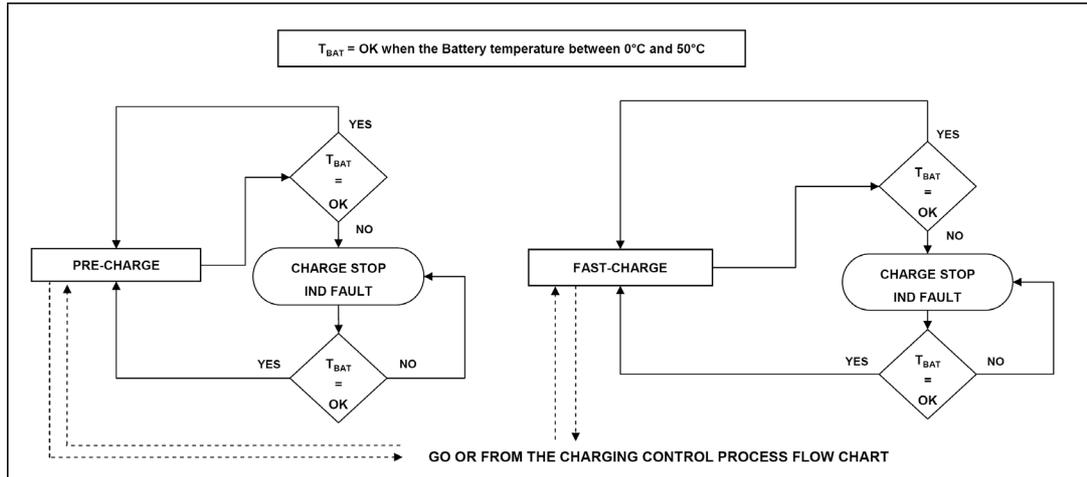
Note:  $T_{BAT} = OK$  when the battery temperature is between 0 °C and 50 °C
