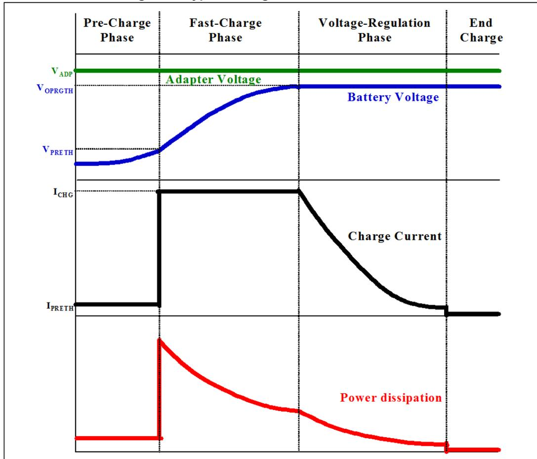
The worst case in power dissipation occurs when the device starts the fast-charge phase. In fact, the battery voltage is at its minimum value. In this case, there is the maximum difference between the adapter voltage and battery voltage, and the charge current is at its maximum value.
