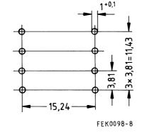
Hole arrangement View in mounting direction
