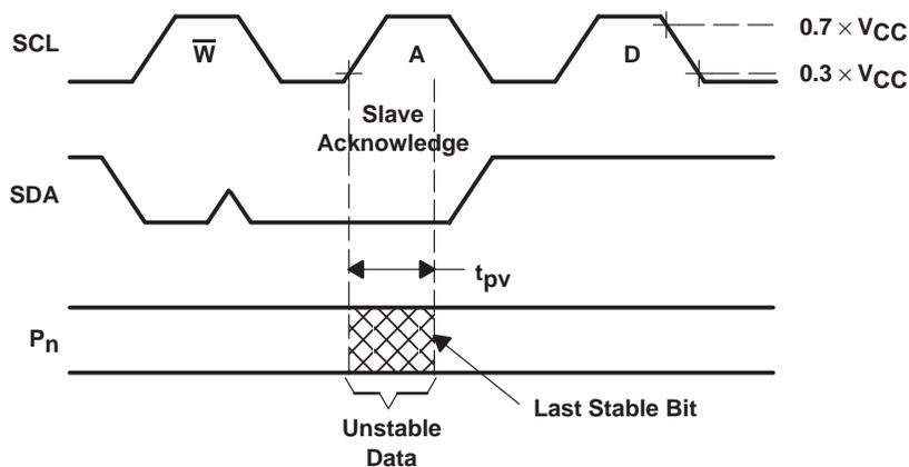
Figure 3. Write-Mode Timing
