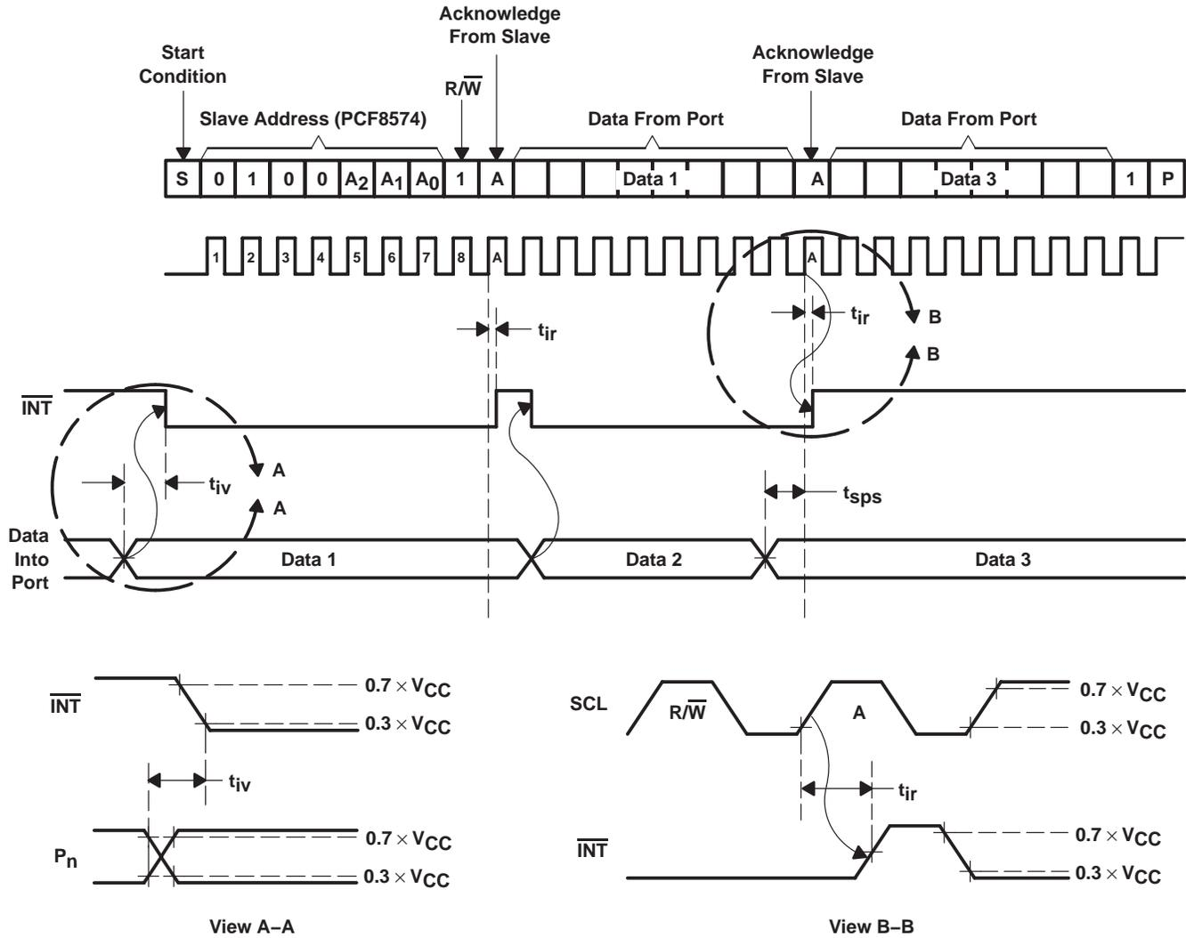
Figure 2. Interrupt-Timing Waveforms
