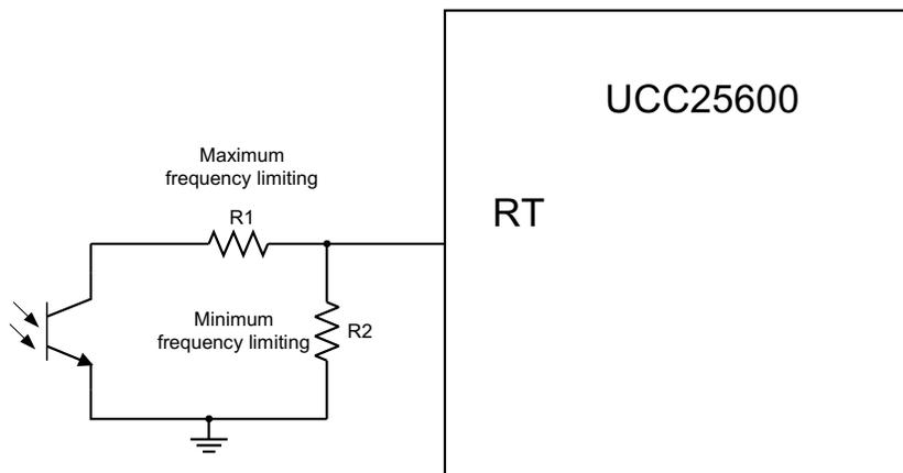
Figure 20. Maximum and Minimum Frequency Setting for UCC25600
