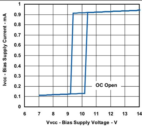
Figure 1. Bias Supply Current vs Bias Supply Voltage
