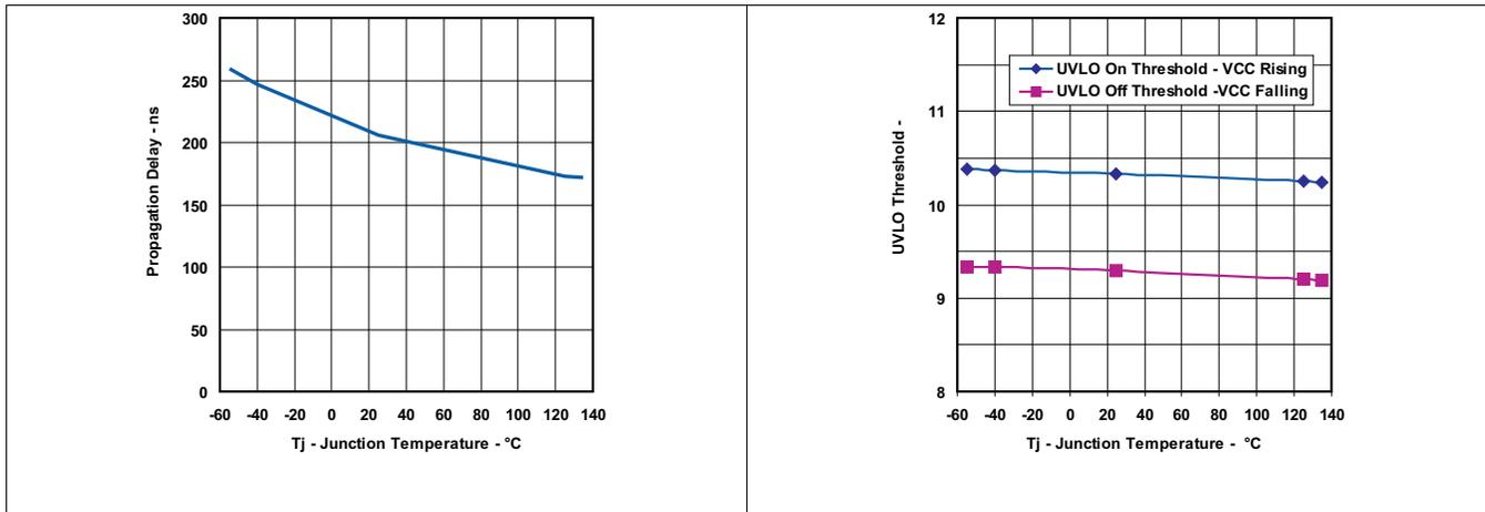
**Figure 7. Overcurrent Propagation Delay vs Temperature**
