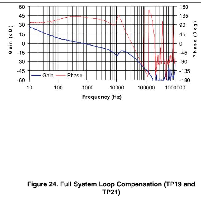
Figure 24. Full System Loop Compensation (TP19 and TP21)
