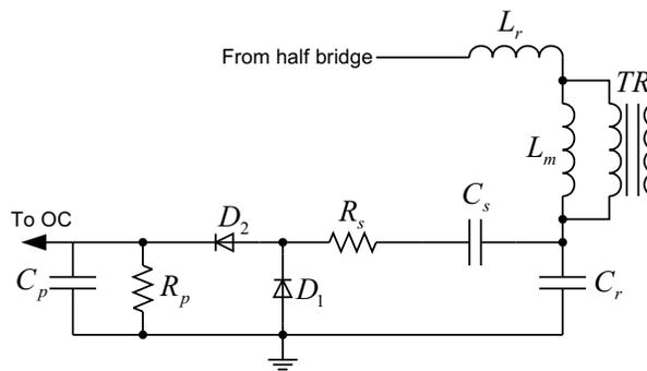
**Figure 13. Current Sensing for LLC Resonant Converter**
