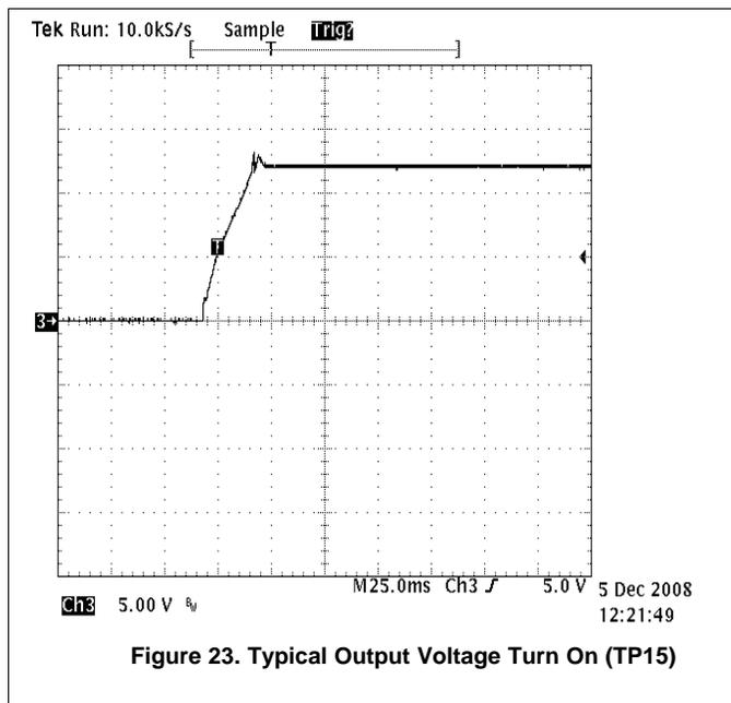
Figure 23. Typical Output Voltage Turn On (TP15)
