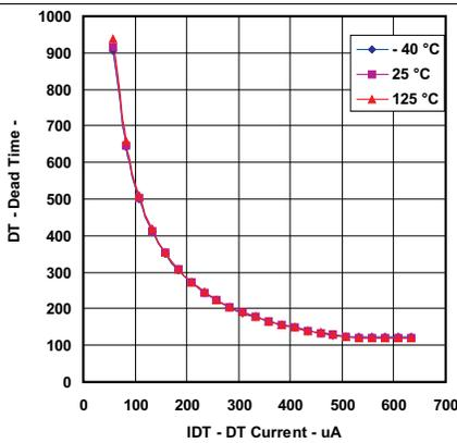
Figure 3. Dead Time vs DT Current
