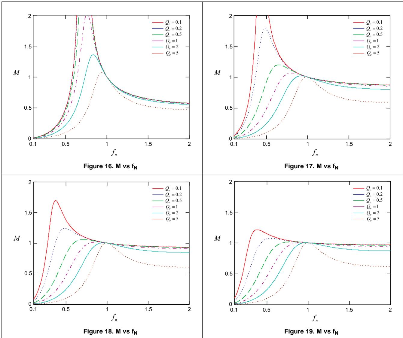
Based on its theory of operation, the LLC resonant converter is controlled through pulse frequency modulation (PFM). The output voltage is regulated by adjusting the switching frequency according to the input and output conditions. Optimal efficiency is achieved at the nominal input voltage by setting the switching frequency close to the resonant frequency. When the input voltage drops low, the switching frequency is decreased to boost the gain and maintain regulation.
