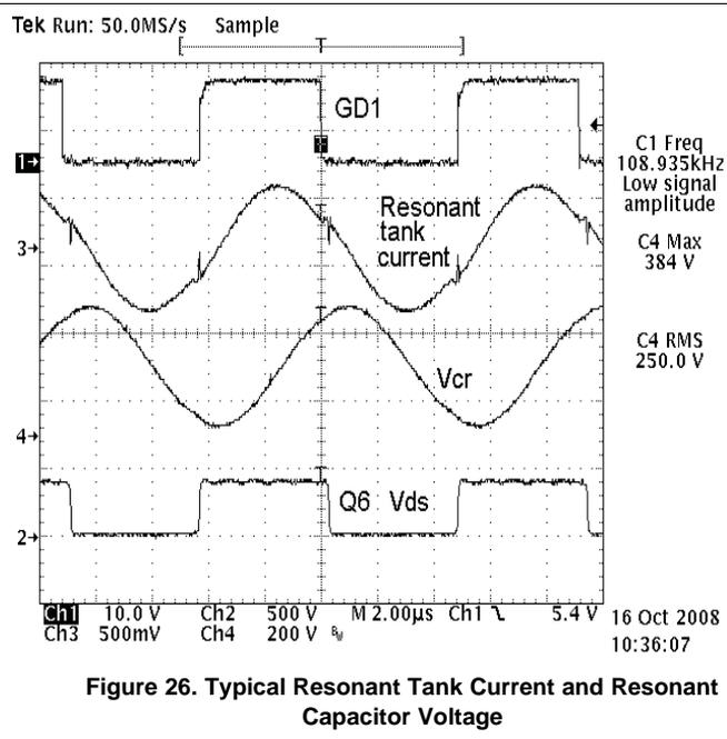
Figure 26. Typical Resonant Tank Current and Resonant Capacitor Voltage
