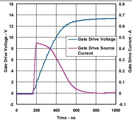
Figure 6. Gate Drive Rising, VCC = 15 V
