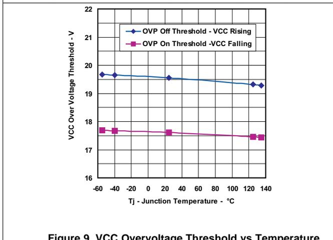
**Figure 9. VCC Overvoltage Threshold vs Temperature**
