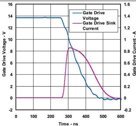
Figure 5. Gate Drive Falling, VCC = 15 V
