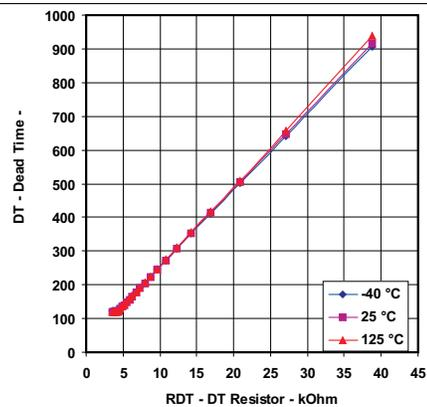
Figure 4. Dead Time vs DT Resistor
