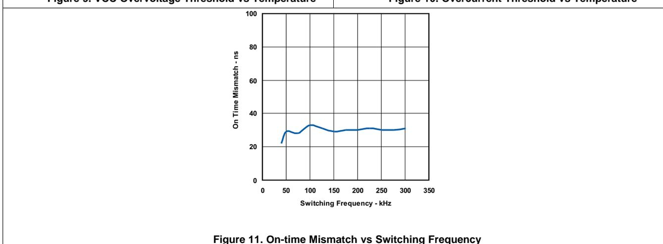
**Figure 11. On-time Mismatch vs Switching Frequency**
