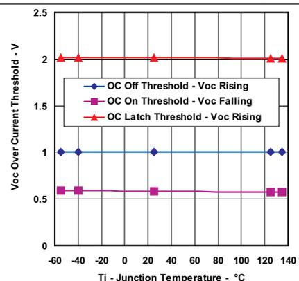
**Figure 10. Overcurrent Threshold vs Temperature**
