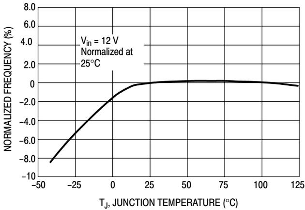
Figure 10. Oscillator Frequency
