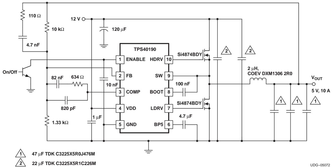
Figure 9. 12-V to 5-V at 10 A
