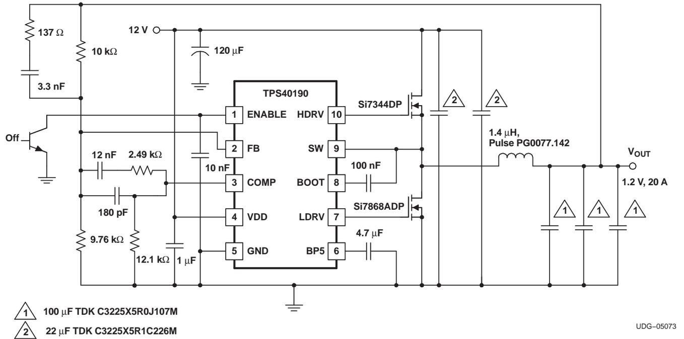
Figure 10. 12-V to 1.2-V at 20 A
