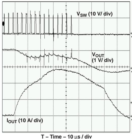
**Figure 1. Output Short Circuit Detected (Nominal Threshold 25 A)**
