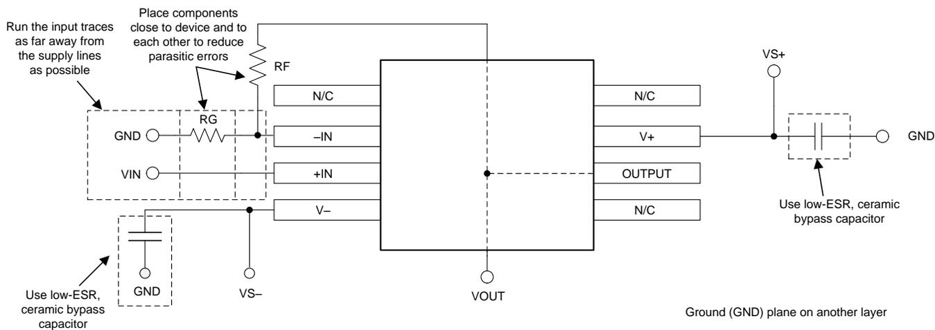
**Figure 33. Operational Amplifier Board Layout for Noninverting Configuration**
