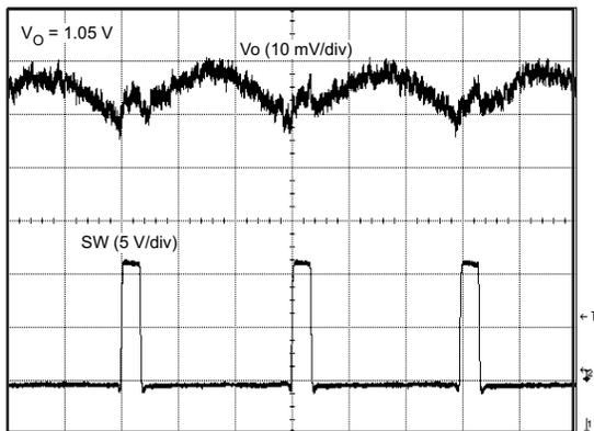
Figure 14. Voltage Ripple vs Ripple at Output ( $I_O = 4\text{ A}$ )
