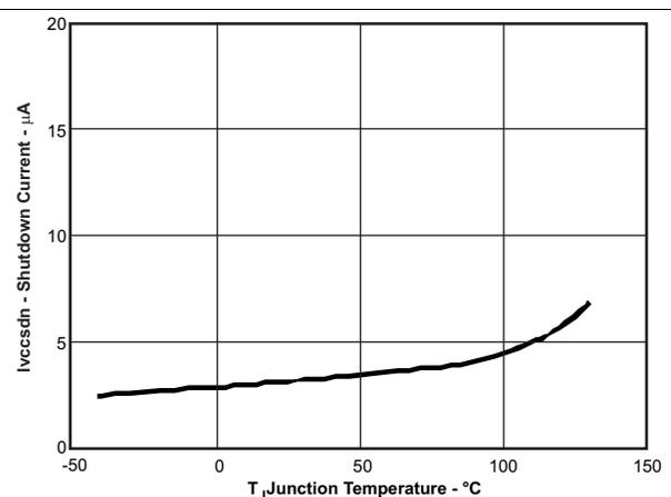
Figure 2. VIN Shutdown Current vs Junction Temperature
