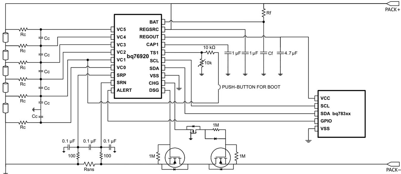
**Figure 2-5. bq76920 with bq783xx Companion Controller IC**
