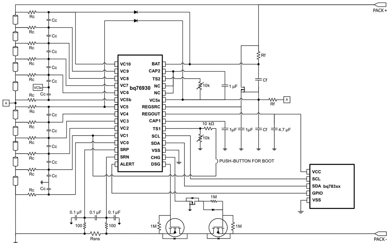
**Figure 2-6. bq76930 with bq783xx Companion Controller IC**
