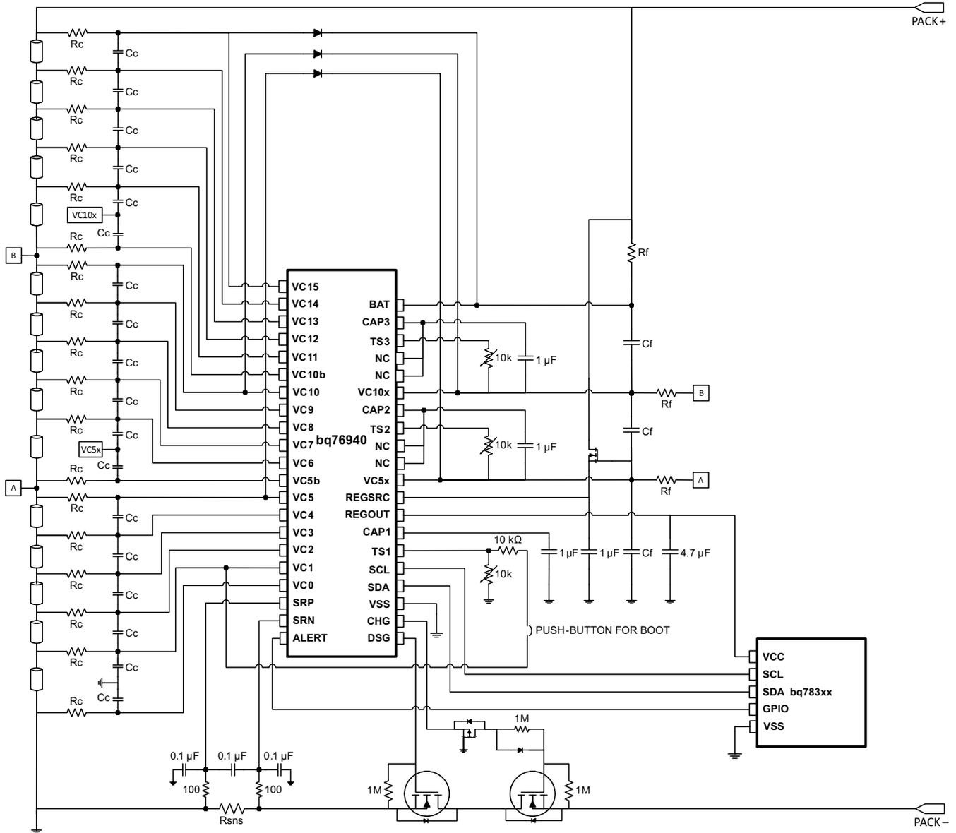
Figure 2-7. bq76940 with bq783xx Companion Controller IC
