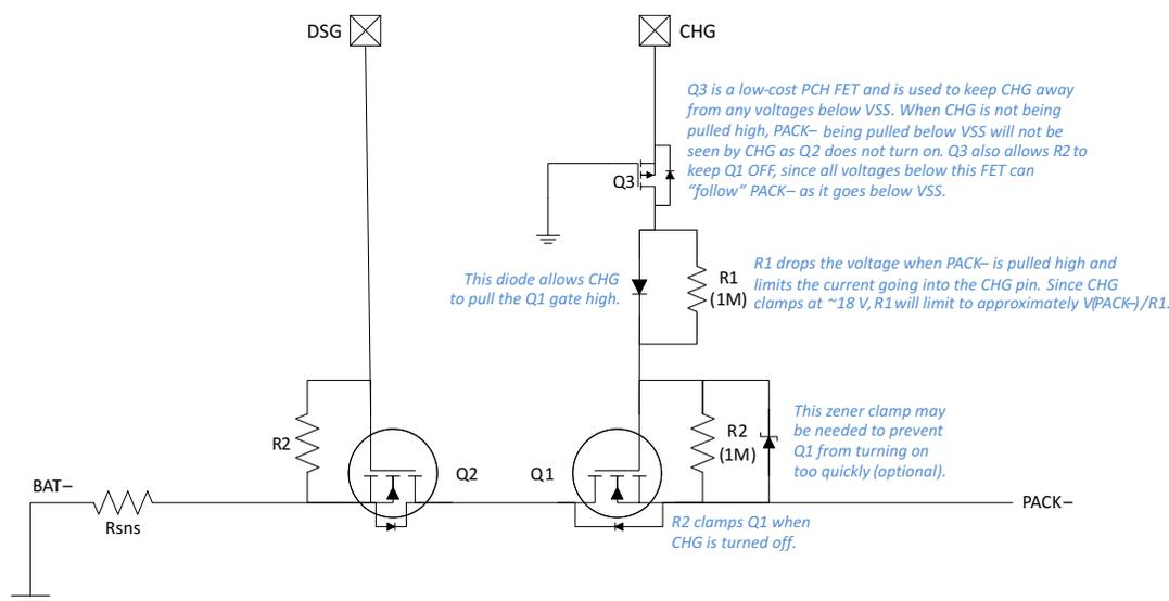
The power path for the CHG and DSG pull-up circuit originates from the REGSRC terminal, instead of BAT.
