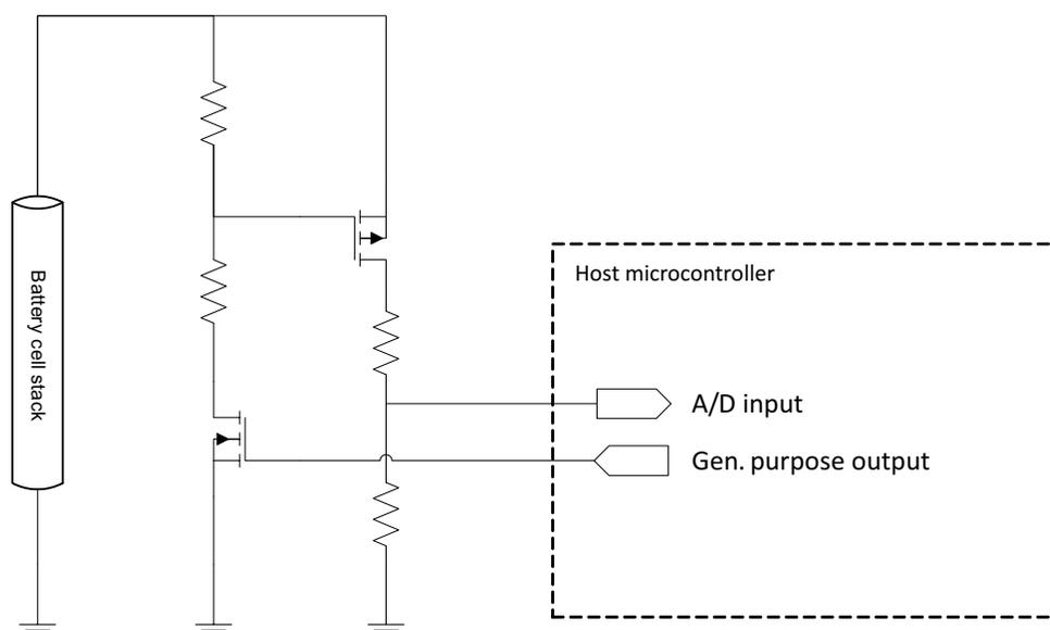
**Figure 5-1. External Real-Time Calibration Circuit to Host Microcontroller**
