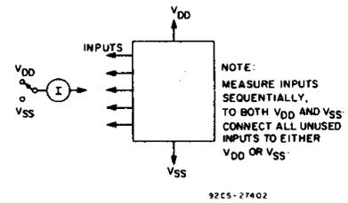
Fig. 13 - Input leakage current test circuit.
