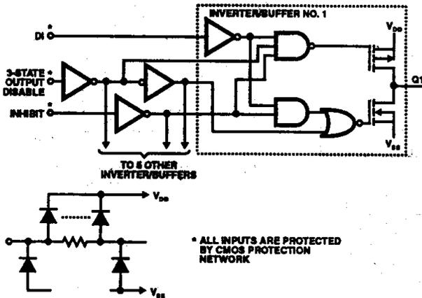
Fig. 1 – Logic diagram of 1 of 6 identical inverter/buffers.
