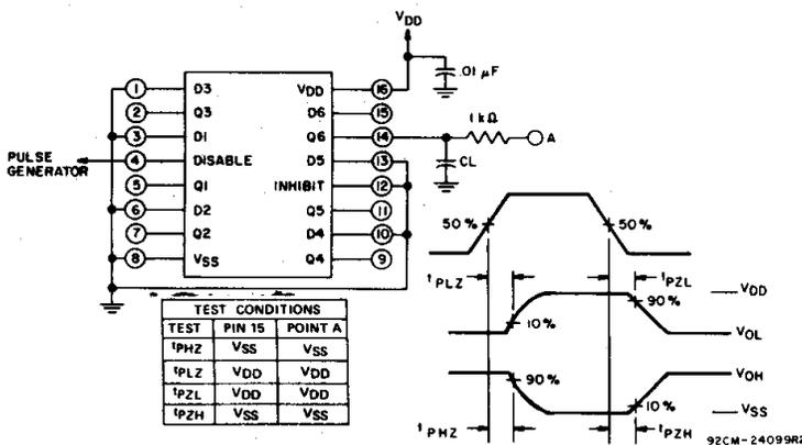
Fig. 14 - Disable delay times test circuit and waveforms.
