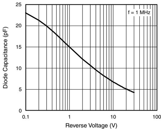
Fig. 5 - Diode Capacitance vs. Reverse Voltage
