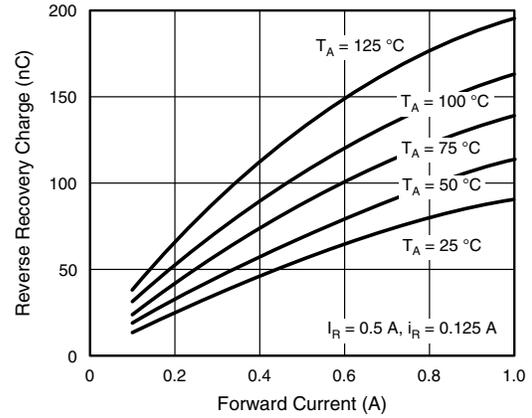
Fig. 6 - Max. Reverse Recovery Charge vs. Forward Current
