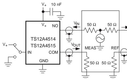
Measurements are standardized against short at socket terminals. OFF isolation is measured between COM and OFF terminals on each switch. ON loss is measured between COM and ON terminals on each switch. Signal direction through switch is reversed; worst values are recorded.
