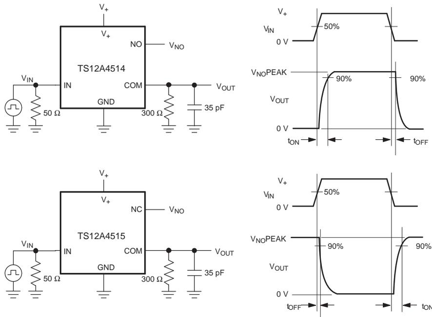
Figure 2. Switching Times
