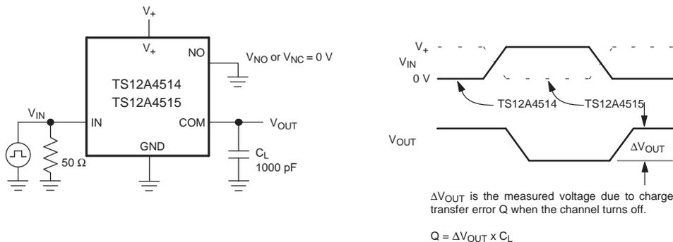
**Figure 1. Charge Injection**
