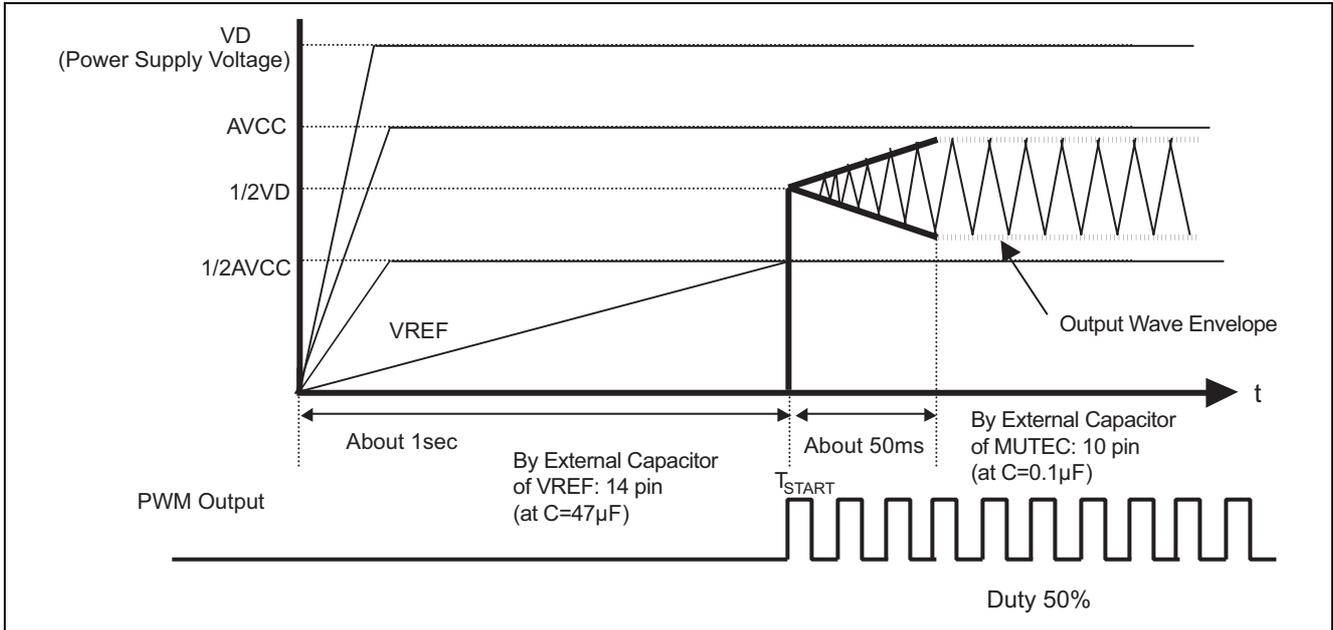
T<sub>START</sub> means the time by reached VREF to 1/2Avcc and determined automatically by the value of capacitor C<sub>REF</sub> connected to external parts according to the following formula.
