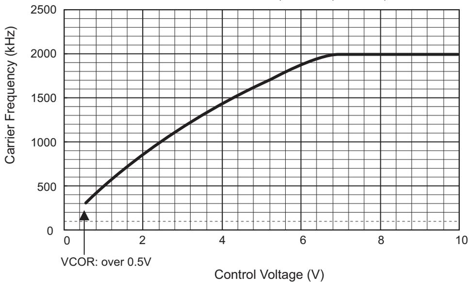
(2) The setting method of Carrier signal I/O
