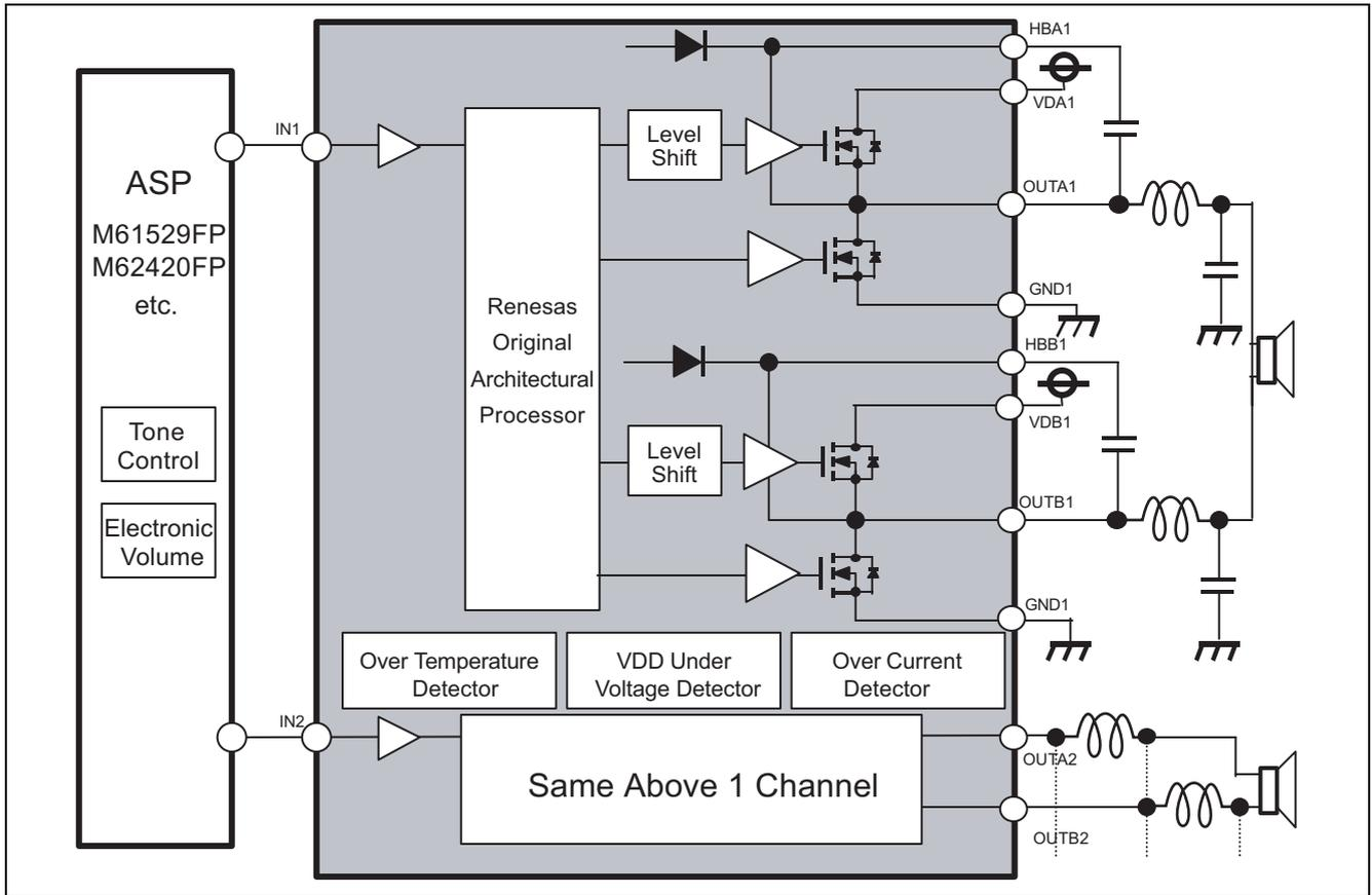
Pin Layout and Internal Block Diagram
