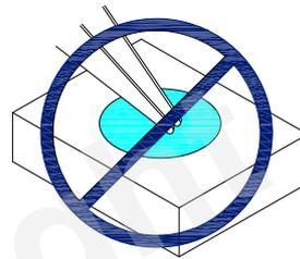
3. Do not stack together assembled PCBs containing exposed LEDs. Impact may scratch the silicone lens or damage the internal circuitry.
