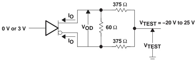
Figure 2. Driver Test Circuit,  $V_{OD}$  With Common-Mode Loading
