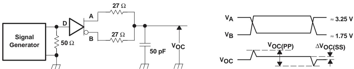
Figure 4. Driver  $V_{OC}$  Test Circuit and Waveforms
