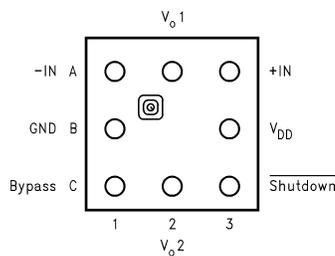
Figure 4. 8-Bump DSBGA - Top View
