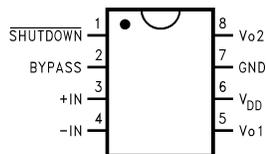
Figure 2. Small Outline (SOIC) Package - Top View
