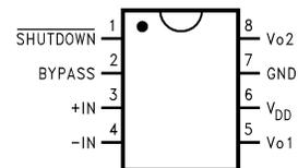
Figure 3. Mini Small Outline (VSSOP) Package – Top View
