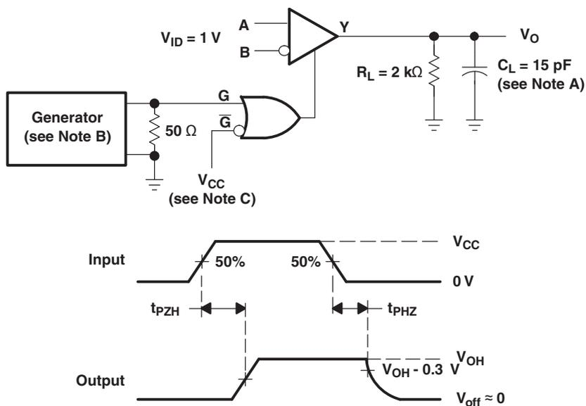
A.  $C_L$  includes probe and jig capacitance.
