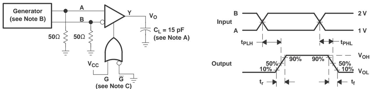
A.  $C_L$  includes probe and jig capacitance.
