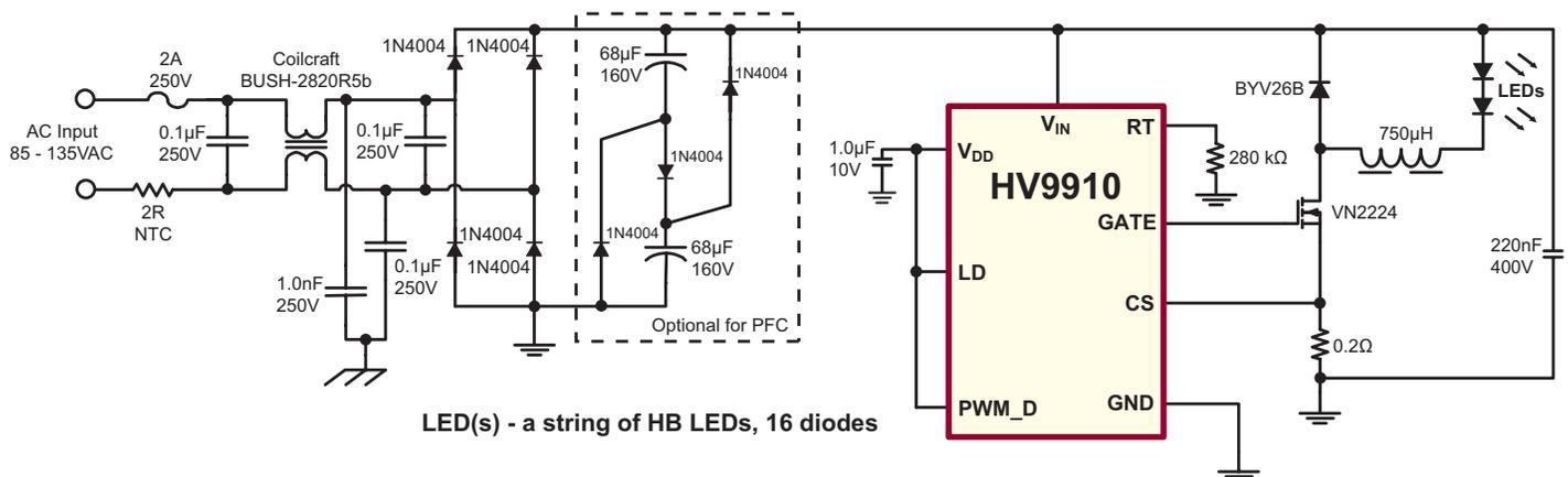
the switching transistor is ON. The energy is then delivered to the output during the OFF time of the transistor. When the energy stored in the Flyback inductor is not fully depleted by the next switching cycle (continuous conduction mode) the DC conversion between input and output voltage is given by:
