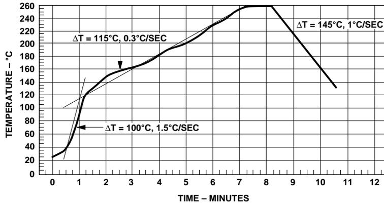
Figure 1. Maximum Solder Reflow Thermal Profile.
