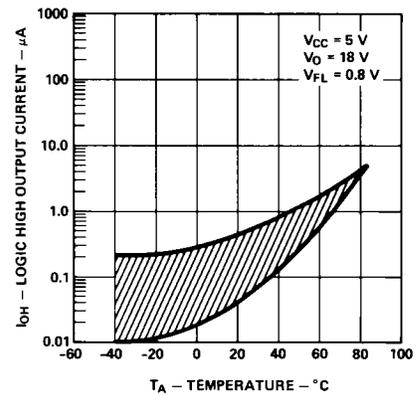
Figure 4. Typical Logic High Output Current vs. Temperature.
