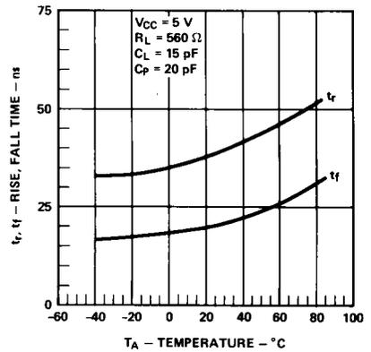
Figure 7. Typical Rise, Fall Time vs. Temperature.
