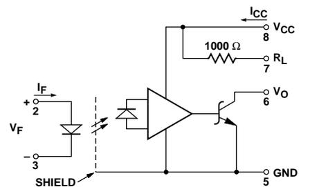
A 0.1  $\mu\text{F}$  CAPACITOR MUST BE CONNECTED BETWEEN PINS 8 AND 5 (SEE NOTE 1).
