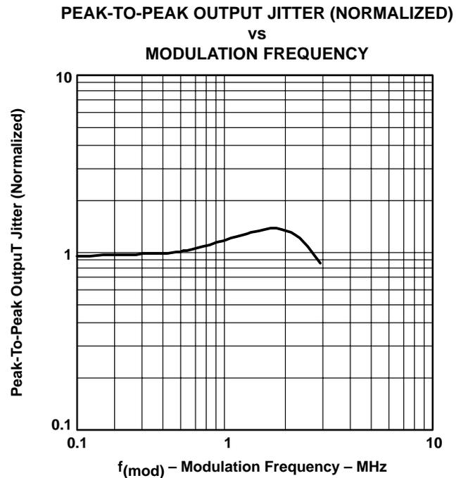
**Figure 11. Output Period Jitter vs Modulation Frequency**
