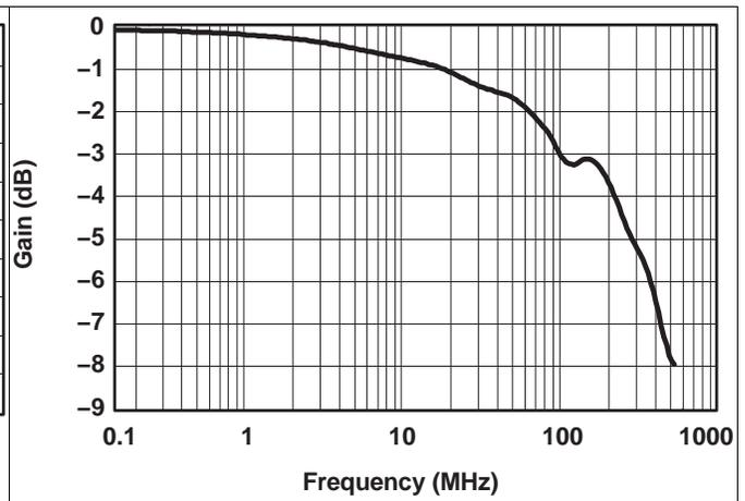
Figure 8. Bandwidth (V<sub>+</sub> = 5 V)
