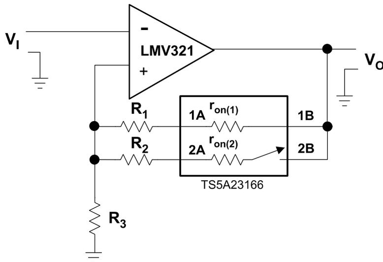
Figure 21. Gain-Control Circuit for OP Amplifier
