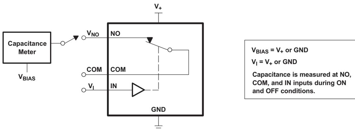
Figure 14. Capacitance ( $C_I$ ,  $C_{COM(OFF)}$ ,  $C_{COM(ON)}$ ,  $C_{NC(OFF)}$ ,  $C_{NC(ON)}$ )
