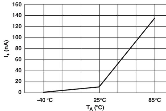
Figure 22. Power-Supply Current vs Temperature (V<sub>+</sub> = 5 V)
