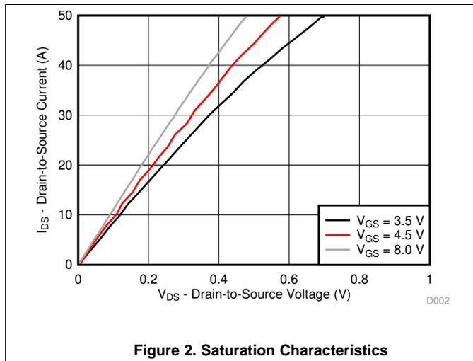
Figure 2. Saturation Characteristics
