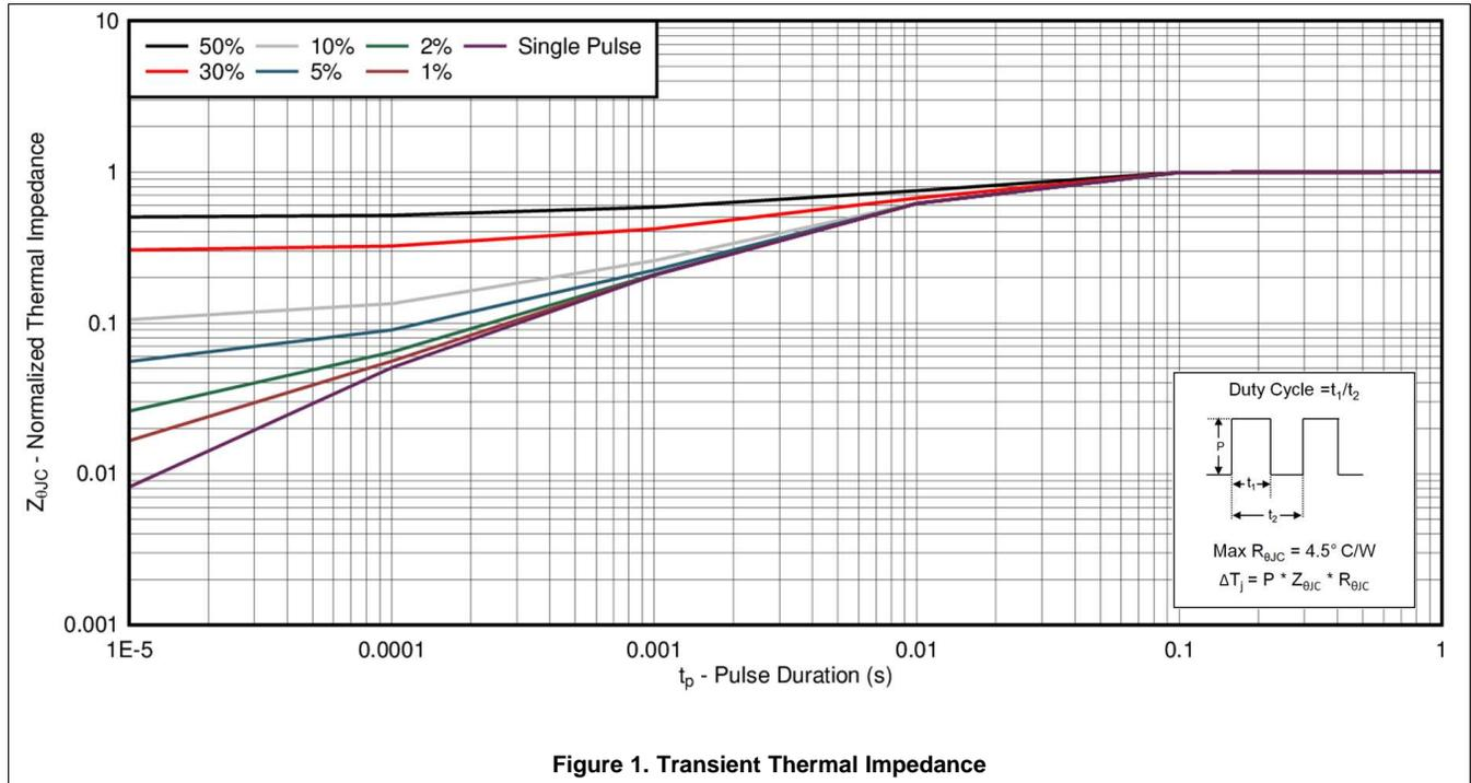
Figure 1. Transient Thermal Impedance
