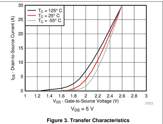
Figure 3. Transfer Characteristics
