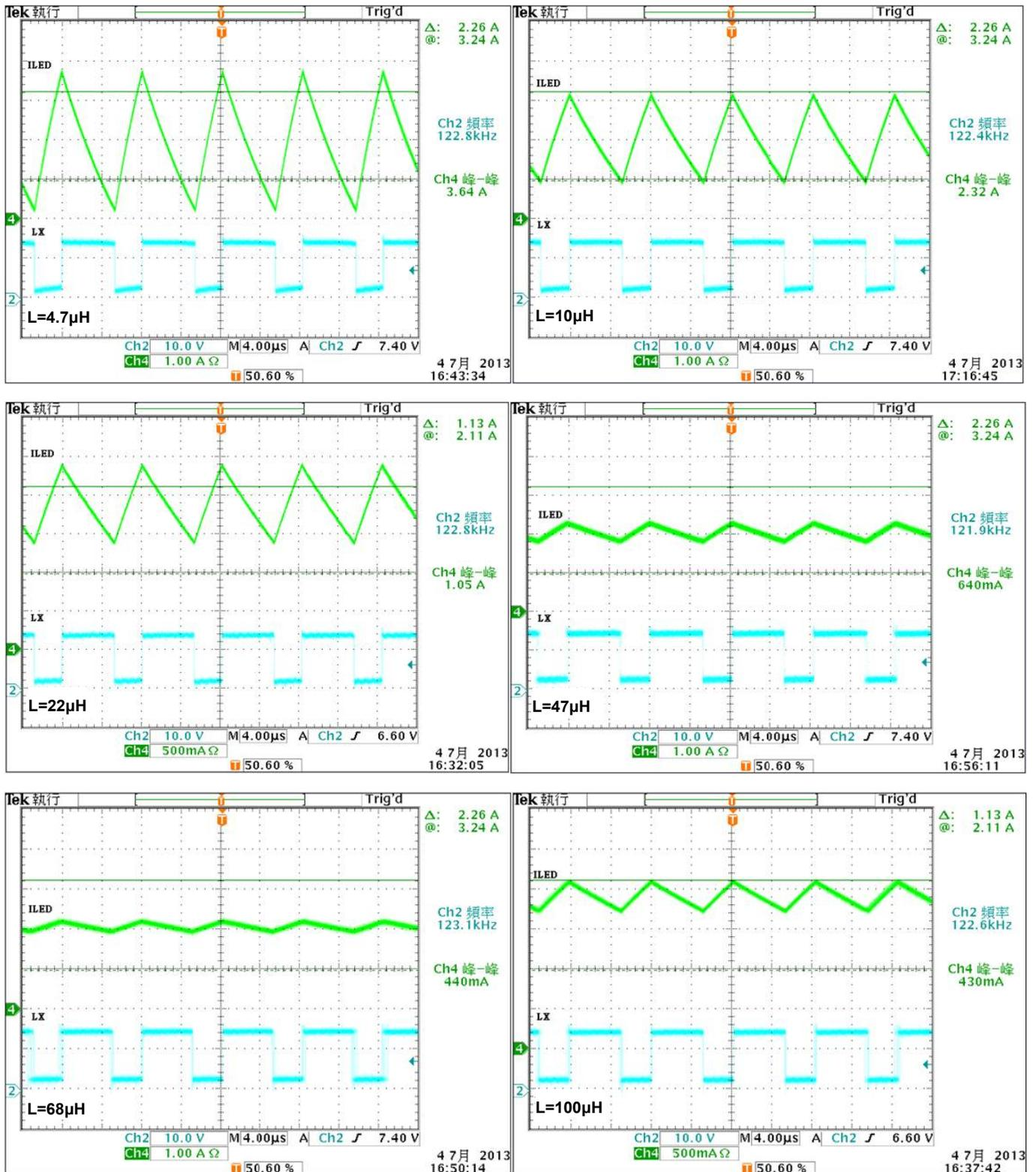
Fig.14 Typical switching waveforms of MBI6662: L=4.7µH~100µH
