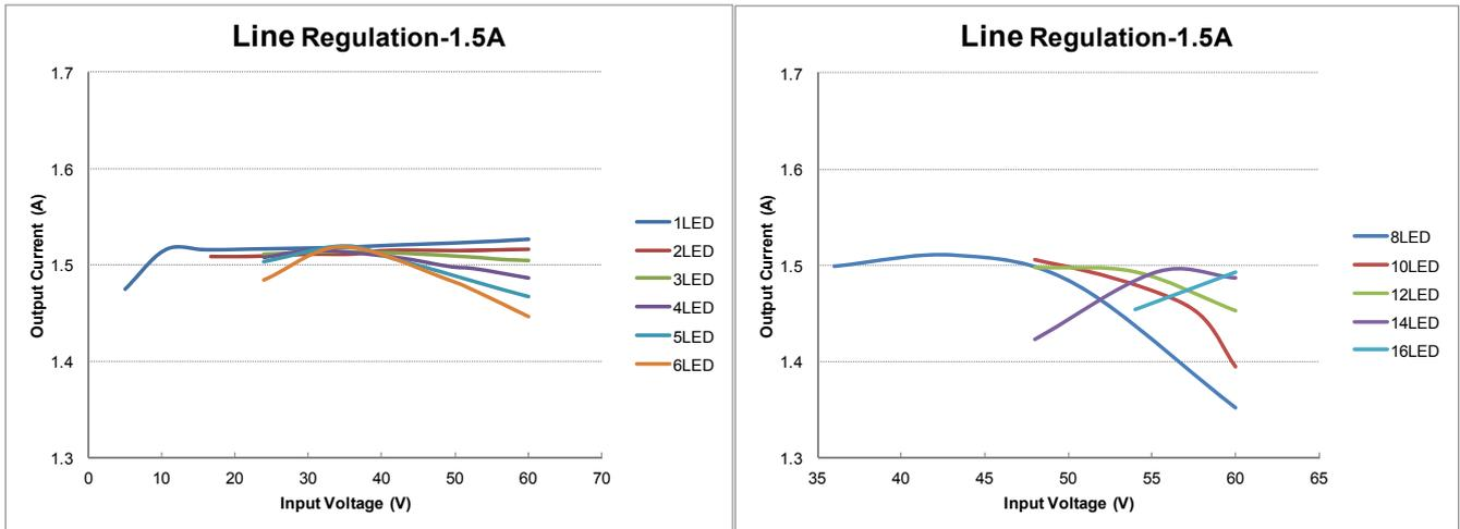
Fig.8 Line regulation of MBI6662: 1.5A output current
