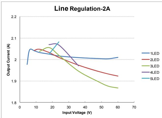
Fig.9 Line regulation of MBI6662: 2A output current
