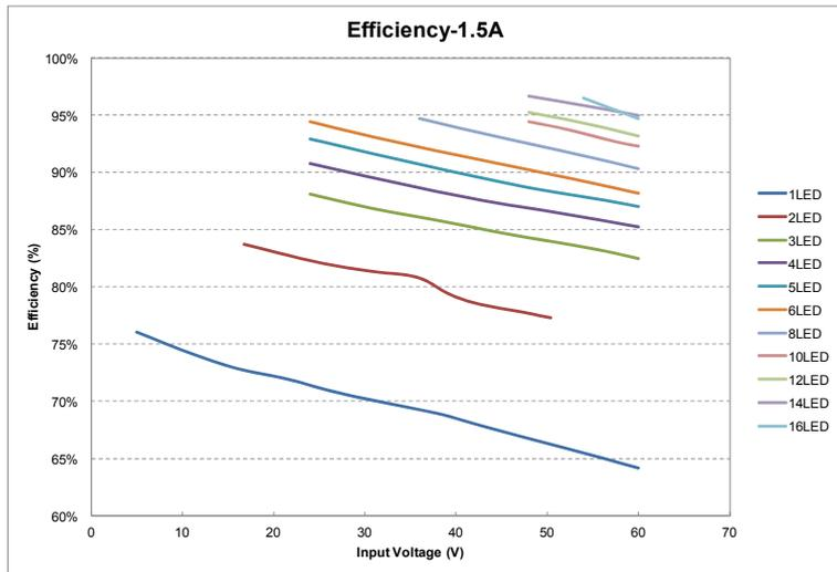
Fig.5 Efficiency of MBI6662: 1.5A output current
