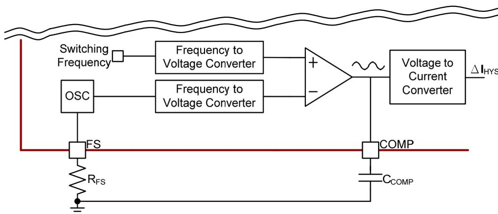
Fig.18 Constant frequency control scheme of MBI6662
