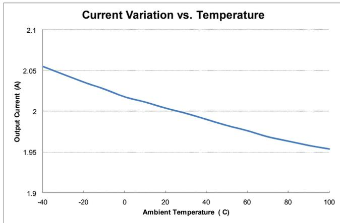
Fig.10 Output current variation with respect to temperature
