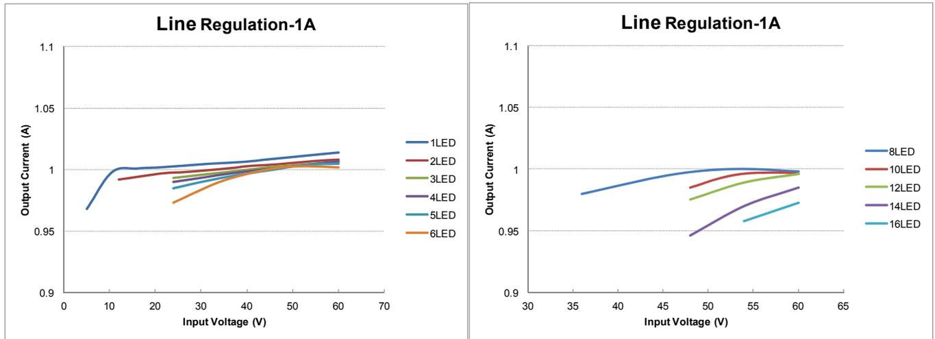
Fig.7 Line regulation of MBI6662: 1A output current
