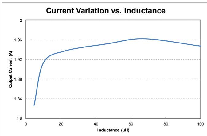
Fig.11 Output current variation with respect to inductance
