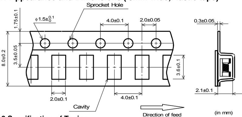
\*Dimension of the Cavity is measured at the bottom side.
