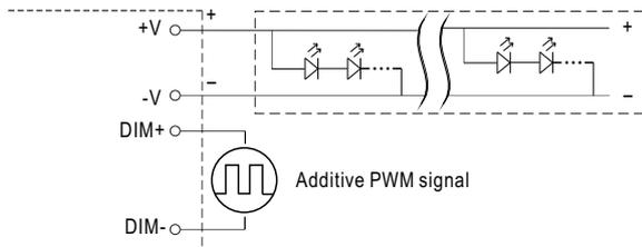
"DO NOT connect "DIM- to -V"
