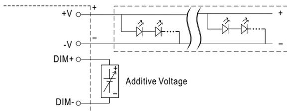
"DO NOT connect "DIM- to -V"
