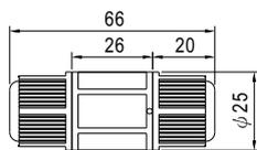
CJ04-1 suitable for 14AWG~16AWG
