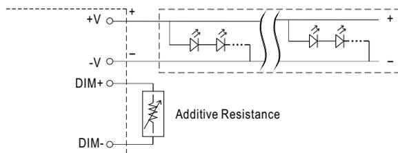
"DO NOT connect "DIM- to -V"
