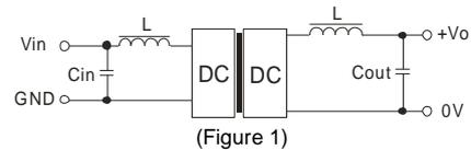
It should also be noted that the inductance and the frequency of the "LC" filtering network should be staggered with the DC/DC frequency to avoid mutual interference. However, the capacitance of the output filter capacitor must be proper. If the capacitance is too big, a startup problem might arise. For every channel of output, provided the safe and reliable operation is ensured, the recommended capacitance of its filter capacitor sees (Table 1).
