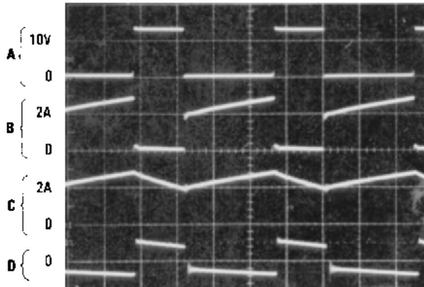
A: Switch pin voltage, 10 V/div
