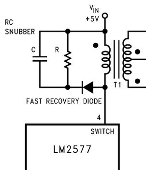
Figure 23. Snubber Circuit
