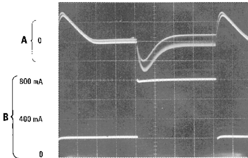
A: Output Voltage Change, 100 mV/div. (AC-coupled)
