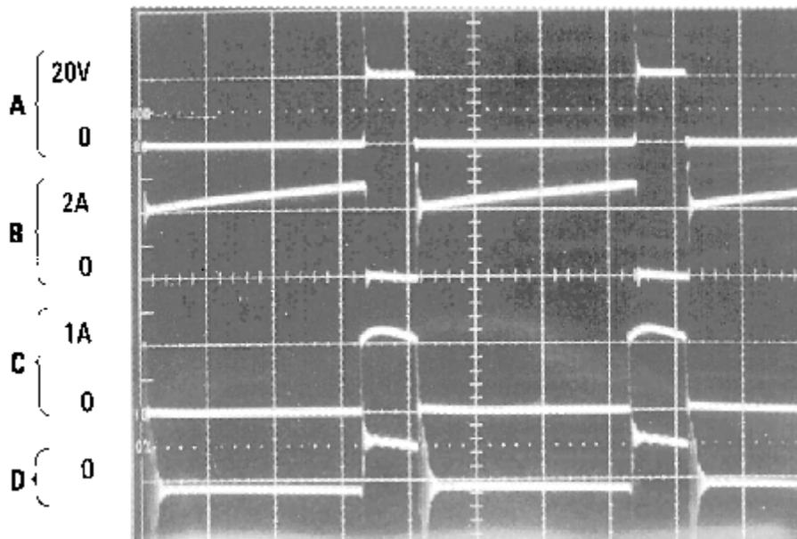
A: Switch pin voltage, 20 V/div
