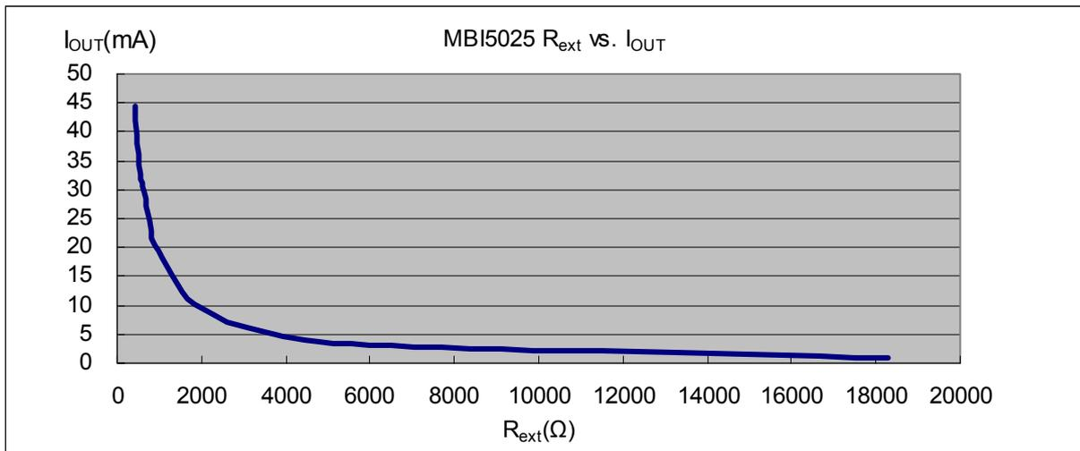
Where  $R_{EXT}$  is the resistance of the external resistor connected to R-EXT terminal and  $V_{R-EXT}$  is the voltage of R-EXT terminal. The magnitude of current (as a function of  $R_{EXT}$ ) is around 25mA at 744 $\Omega$  and 10mA at 1860 $\Omega$ .
