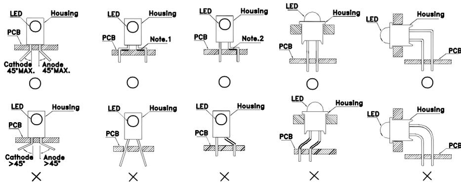
”○” Correct mounting method ”×” Incorrect mounting method
