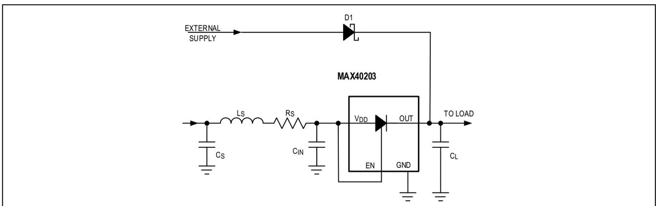
Figure 3. Typical OR Application Showing Source Impedance
