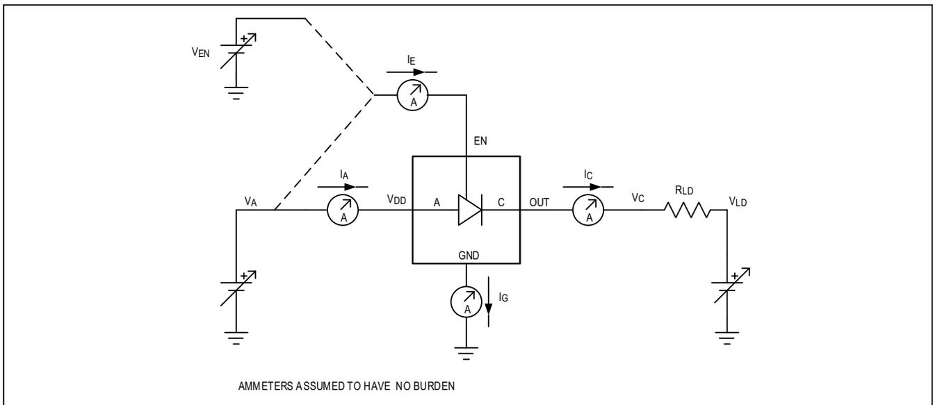
Figure 2. Ideal Diode Test Setup and Naming Convention
