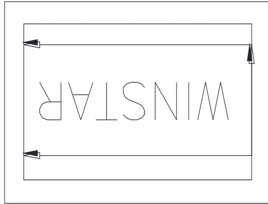
Fig. 1 Normal scan ( pin 4, LR/UD = High or NC )
