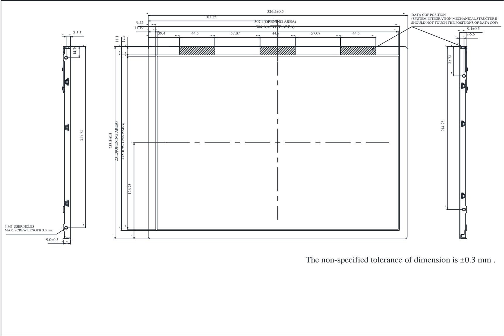
The non-specified tolerance of dimension is ±0.3 mm .
