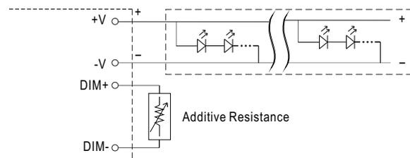
"DO NOT connect "DIM- to -V"
