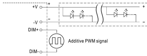
"DO NOT connect "DIM- to -V"
