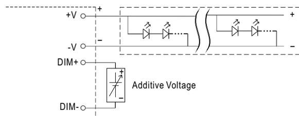
"DO NOT connect "DIM- to -V"
