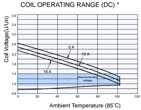
**Notes:** \* The use of a relay with an energising voltage other than the rated coil voltage may lead to reduced electrical life. An energising voltage over the abver range may damage the insulation of relay coil.
