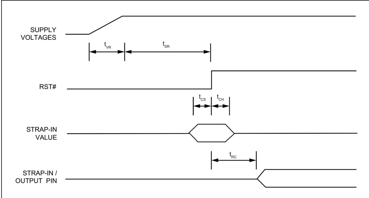
**TABLE 7-5: POWER-UP/RESET TIMING PARAMETERS**
