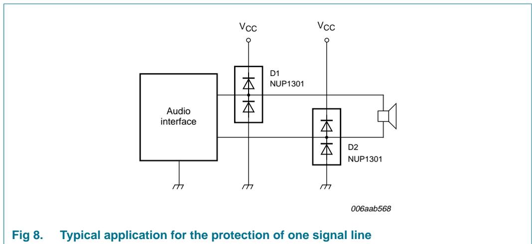
**Fig 8. Typical application for the protection of one signal line**
