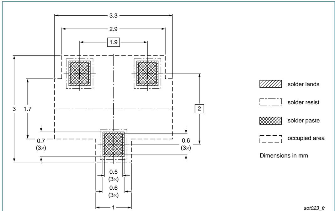
Fig 10. Reflow soldering footprint SOT23 (TO-236AB)
