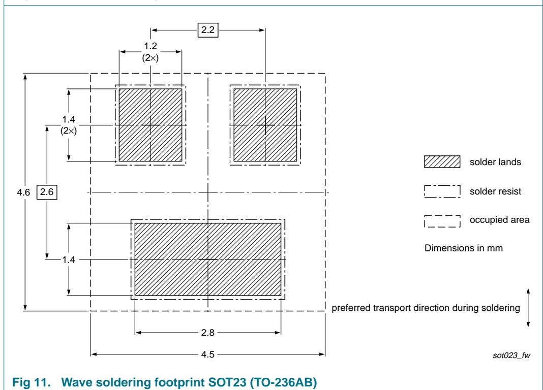
Fig 11. Wave soldering footprint SOT23 (TO-236AB)
