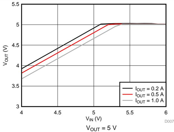
Figure 7. Dropout Curve
