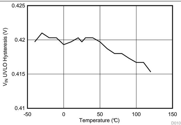
Figure 11.  $V_{IN}$  UVLO Hysteresis vs Junction Temperature
