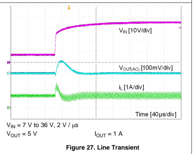
Unless otherwise specified the following conditions apply:  $V_{IN} = 12\text{ V}$ ,  $f_{SW} = 400\text{ kHz}$ ,  $L = 22\text{ }\mu\text{H}$ ,  $C_{OUT} = 47\text{ }\mu\text{F} \times 2$ ,  $T_A = 25^\circ\text{C}$ .
