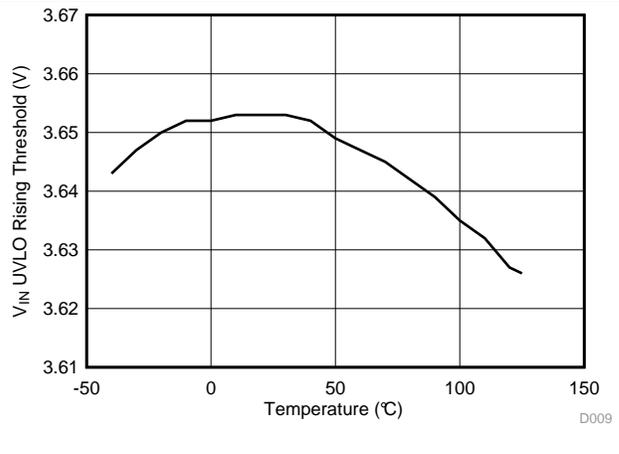
Figure 10.  $V_{IN}$  UVLO Rising Threshold vs Junction Temperature
