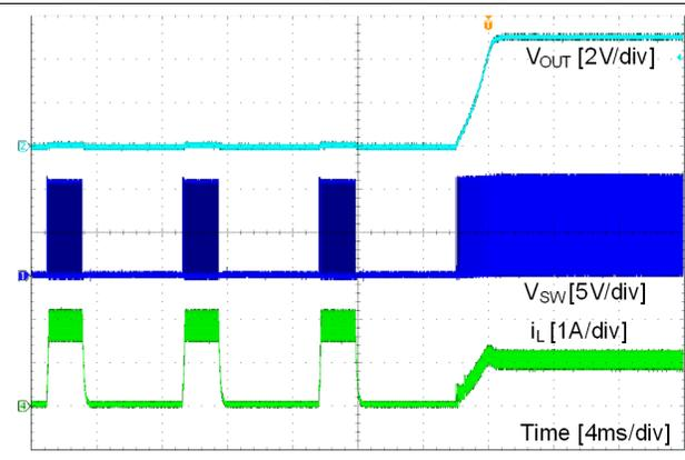
$V_{OUT} = 5\text{ V}$      $I_{OUT} = \text{short to } 1\text{ A}$
