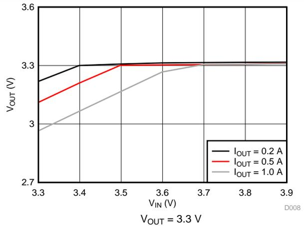
Figure 8. Dropout Curve
