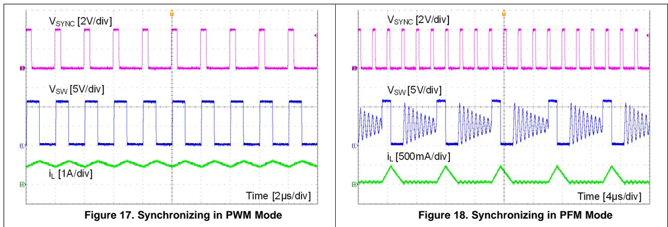
**Figure 17. Synchronizing in PWM Mode**
