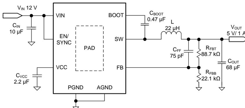
Figure 21. Application Circuit
