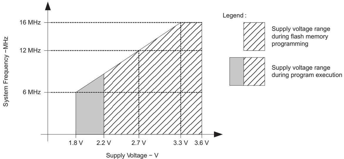
NOTE: Minimum processor frequency is defined by system clock. Flash program or erase operations require a minimum  $V_{CC}$  of 2.2 V.
