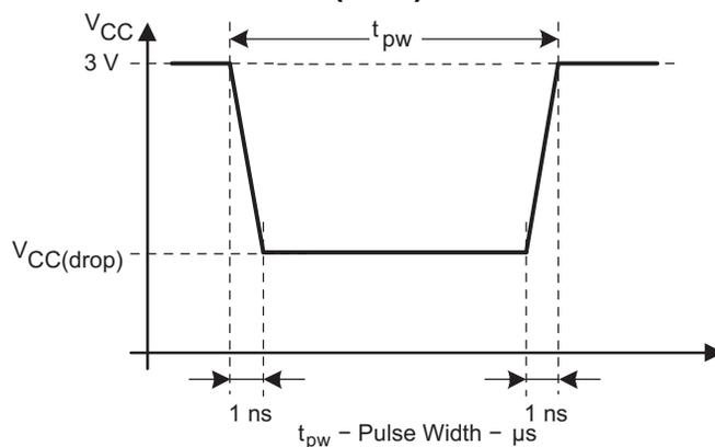
Figure 9. V<sub>CC(drop)</sub> Level With a Square Voltage Drop to Generate a POR/Brownout Signal
