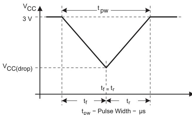
Figure 10. V<sub>CC(drop)</sub> Level With a Triangle Voltage Drop to Generate a POR/Brownout Signal
