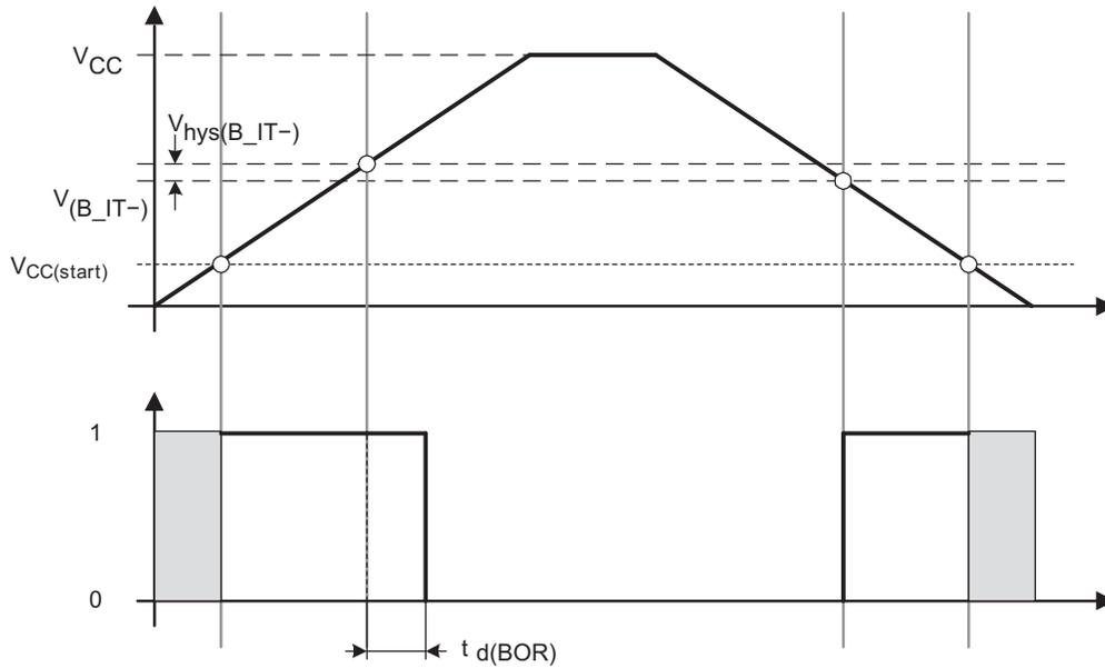
**Figure 8. POR/Brownout Reset (BOR) vs Supply Voltage**
