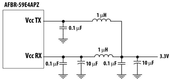
Note: Inductors should have less than 1Ω series resistor per MSA.
