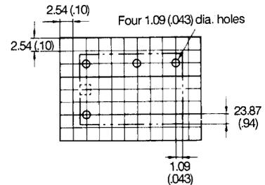
Note: [Hatched box] and [Dashed box] indicate mounting orientation marks.
