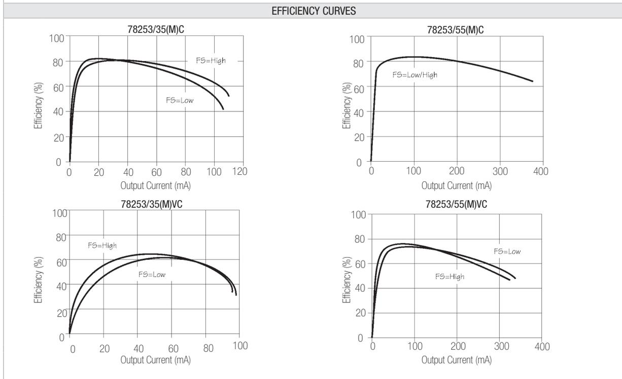
All curves are derived from testing with the Maxim MAX235 IC using the circuit shown in application note MPAN-03 (download at <http://www.murata-ps.com/data/apnotes/mpan-03.pdf>).
