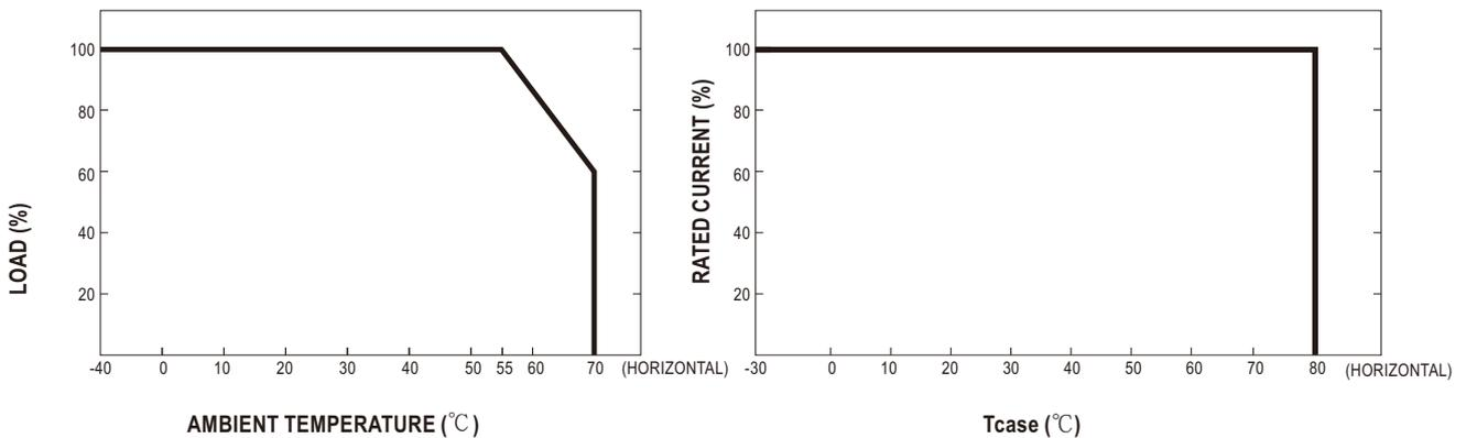
Suitable installation methods are shown as below. Since RSD-150 is a semi-potted model, its thermal performances for the following installation methods are similar and share the same derating curve.
