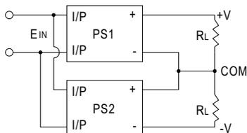
2. Increase the output voltage (current does not change). Because RSD-100 series have no reverse blocking diode in the unit, you should add an external blocking diode to prevent the damage of every unit while starting up. The voltage rating of the external diode should be larger than  $V1+V2$  (as shown as below).
