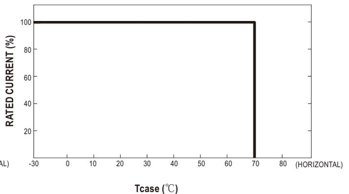
Suitable installation methods are shown as below. Since RSD-100 is a semi-potted model, its thermal performances for the following installation methods are similar and share the same derating curve.
