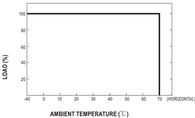
Suitable installation methods are shown as below. Since RSD-100 is a semi-potted model, its thermal performances for the following installation methods are similar and share the same derating curve.
