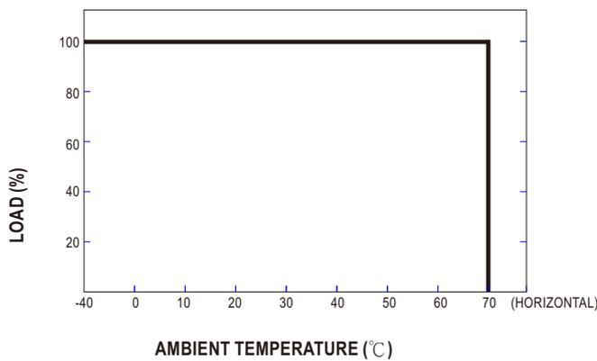
Suitable installation methods are shown as below. Since RSD-200 is a semi-potted model, its thermal performances for the following installation methods are similar and share the same derating curve.
