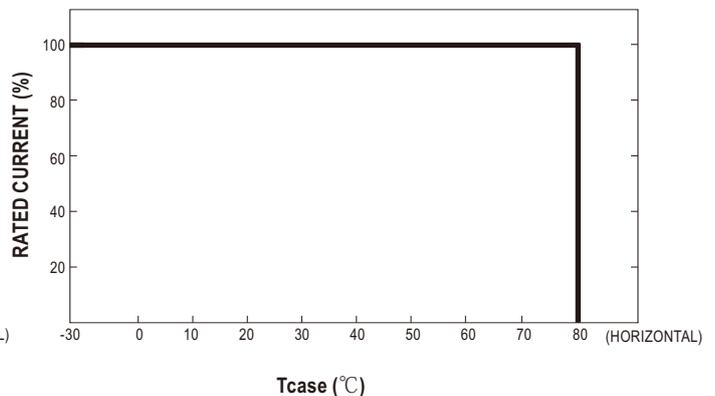
Suitable installation methods are shown as below. Since RSD-200 is a semi-potted model, its thermal performances for the following installation methods are similar and share the same derating curve.
