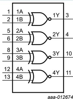
Fig. 1. Functional diagram
