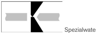
The life time of the cutting tips depend among others on the sharpness. The sharper the tip (Ultra Flush) the faster the wear. Out of this reason pliers in Semi Flush or Flush are preferable so far no ultra flush and shock reduced cut is necessary.
